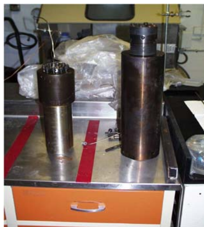
FIGURE 2. Bridgeman seal-type pressure vessel for 300°C, 150 bar hydrothermal experiment.
