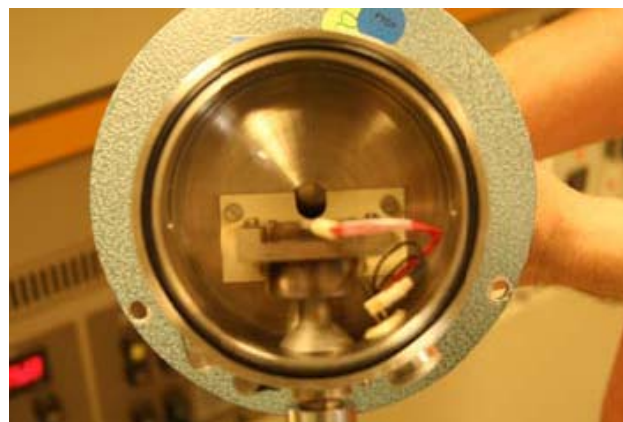
FIGURE 1. XRD cell used for in situ XRD examination under controlled temperature and relative humidity.
