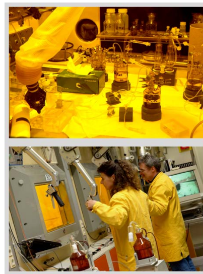
Fig. 1: HLW material is investigated at the Institute for Nuclear Waste Disposal (INE) at KIT. Above: SNF leaching experiments. Below: hot-cell facility at KIT-INE.
